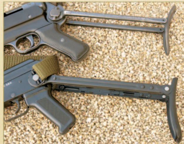
Mikhail Kalashnikov clearly took the down-folder buttstock on the AK47 from the German MP40 submachine gun. It has been carried and used in all corners of the world.
