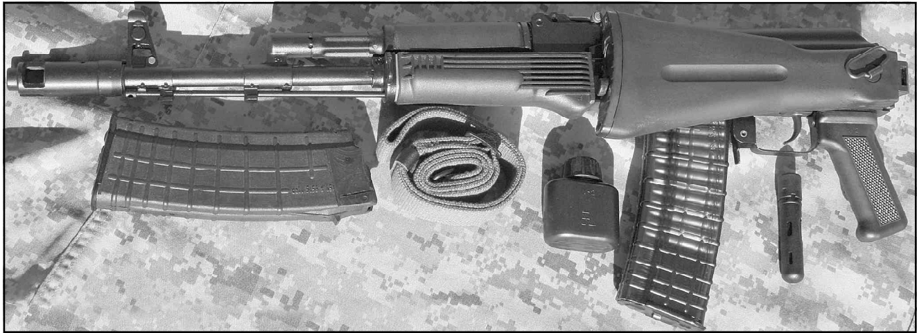
Above: The SLR-106FR with the stock folded and secured. Even with the muzzle brake installed the overall length is reduced by almost 10 inches, from 36.875 inches to a mere 27.375 inches in length.
