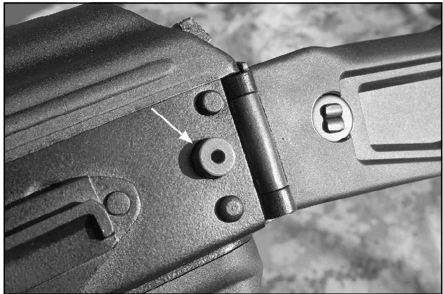
Above: The arrow indicates the buttstock latch that must be depressed to allow the stock to fold. The stock locks very tight in its open position and provides a sturdy and comfortable platform for shooting.
