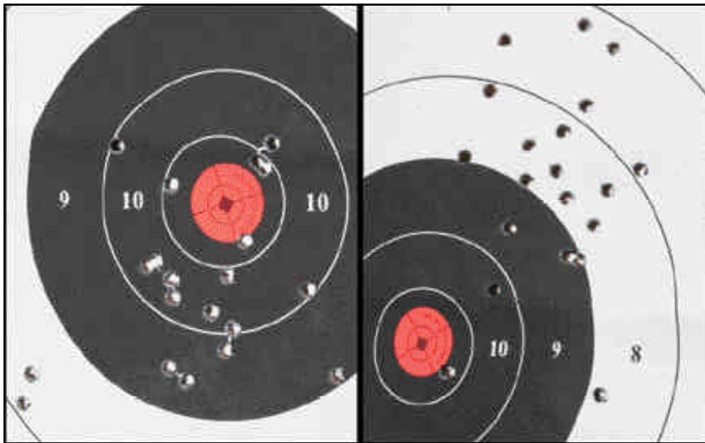
The target on the left is a 20-round group of 62-grain Wolf Polyformance ammo fired in a rapid-fire session with the open, factory sights, at a distance of 50 yards with the SLR-106FR rifle and its 16.25 inch barrel. The target on the right is a 20-round group of 62-grain Wolf Polyformance ammo fired in a rapid-fire session with the open, factory sights at a distance of 50 yards with the SLR-106CR rifle and its 12.5 inch barrel. After the shooting had concluded it was noticed that the sights on the 106CR had inadvertently been set to 200 meters instead of the 100-meter setting. That may explain why the group was a little higher than the point of aim. The orange dot was the point of aim for both strings.
