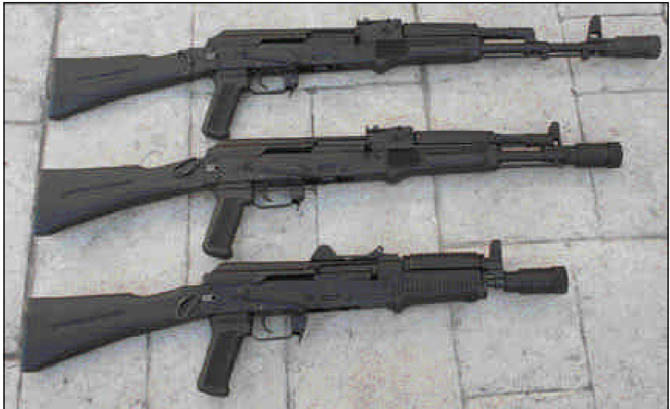
Below: An SLR-106 family portrait. On top is the 106F with a 16.25-inch barrel. In the center is the 106C with a 12.5-inch barrel. On the bottom is the 106U with an 8.5-inch barrel. All models have a standard Bulgarian 24mm thread that will accept a number of available muzzle accessories and are pictured here with the popular 4-piece muzzle brake.
