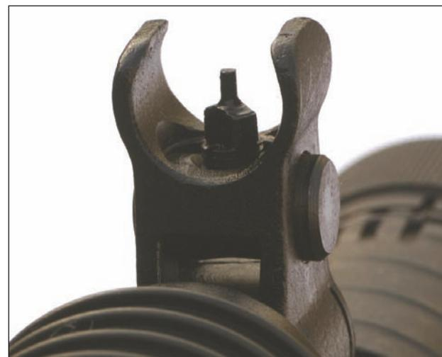
**The standard Kalashnikov-type front sight post, with the usual protective ears, is adjustable for windage and elevation zero providing the proper tools are used.**
