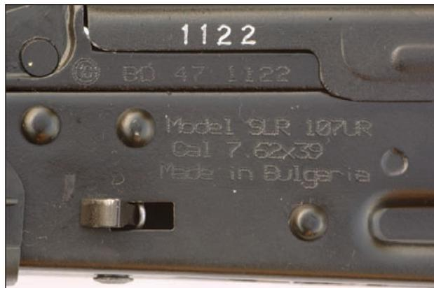
**Both of the available stocks fold to the left and are retained by a spring-loaded locking latch protruding from a rectangular slot in the left side receiver wall.**
