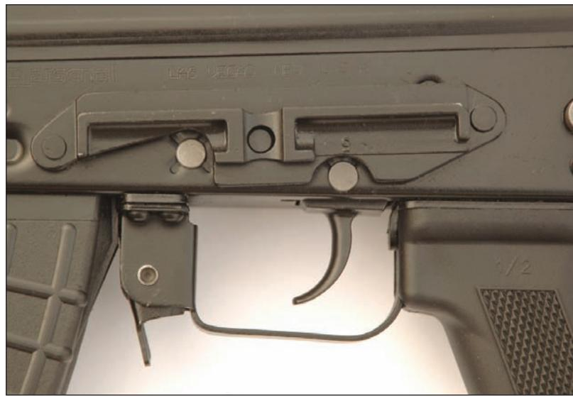
**The pistol grip found on SLR-106 and SLR-107 series rifles is somewhat shallower than the old style and is designed to fit flush with the grip reinforcement plate.**
